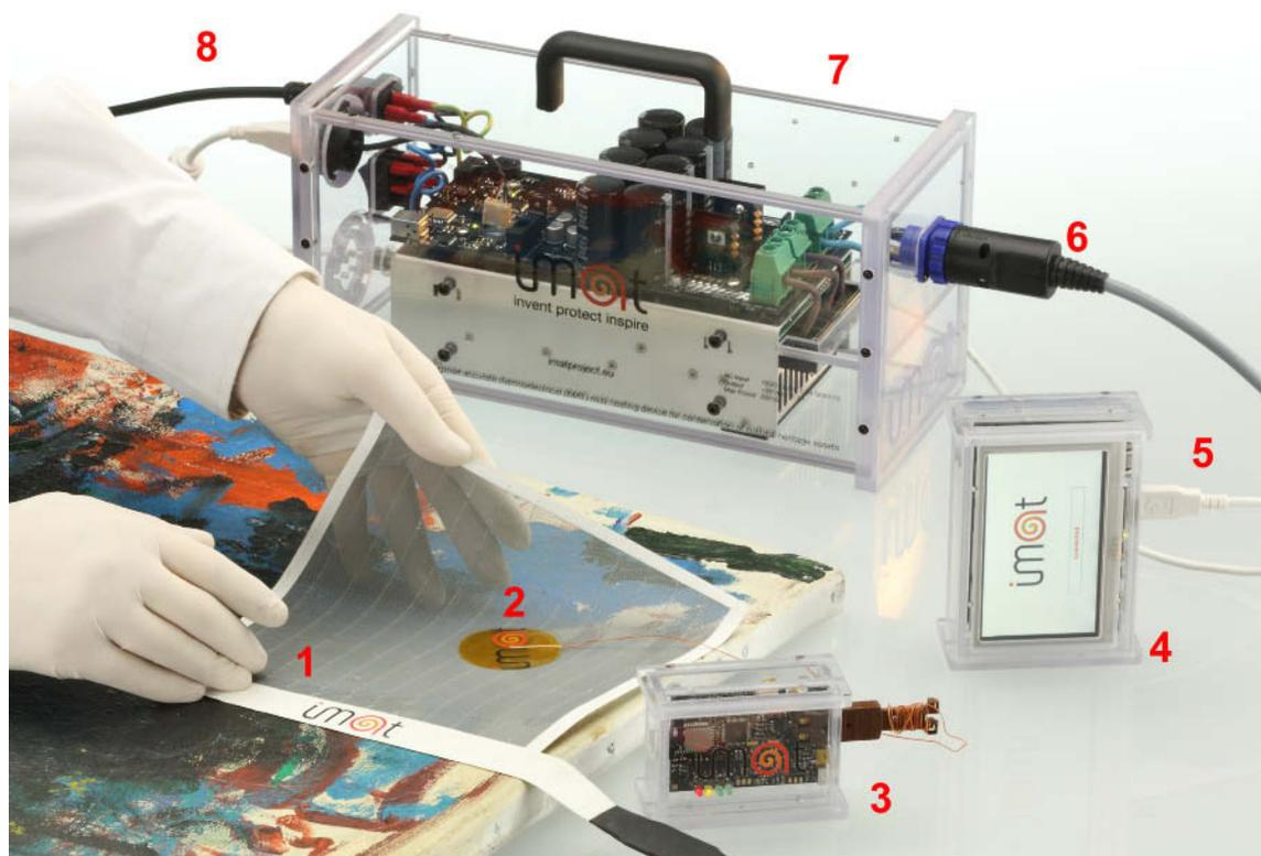
Figure 1. Components of the IMAT mild heat transfer instrument: (1) breathable heater, (2) temperature sensor (thermocouple), (3) wireless temperature sensor, (4) touch screen pad, (5) USB cable, (6) power out cable 36 V, (7) temperature controller, (8) power cable in 120/230 V.
